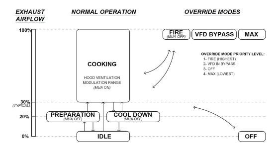
When exhaust dampers are used in combination with an exhaust fan, they are forced to operate according to their corresponding exhaust fan operating mode. This ensures that the exhaust duct air velocity, under cooking conditions, is above 500 ft/min as prescribed by NFPA 96<sup>3</sup>.
